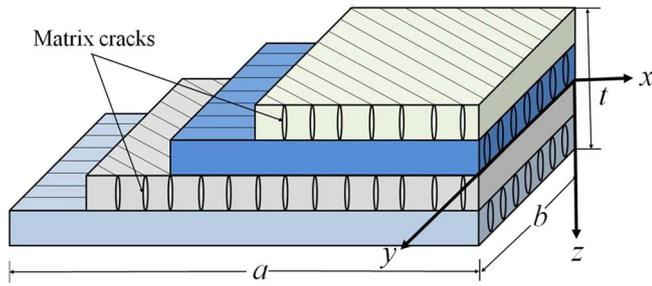
Fig. 1. Configuration of a hybrid matrix crack laminated composite plate composed of perfectly bonded CNTR-FG layers and FRC layers.
