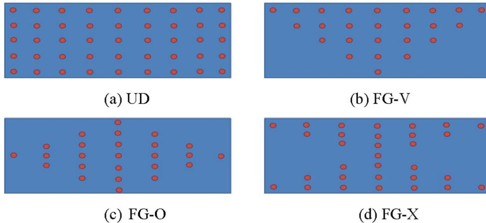
Fig. 2. CNT distributions in CNTR-FG layer.
