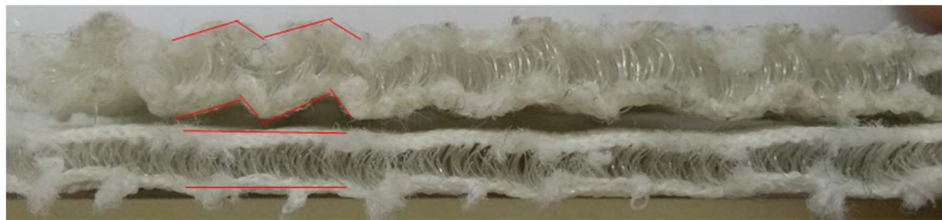
Fig. 2. Comparison lateral view of fabric structures.
