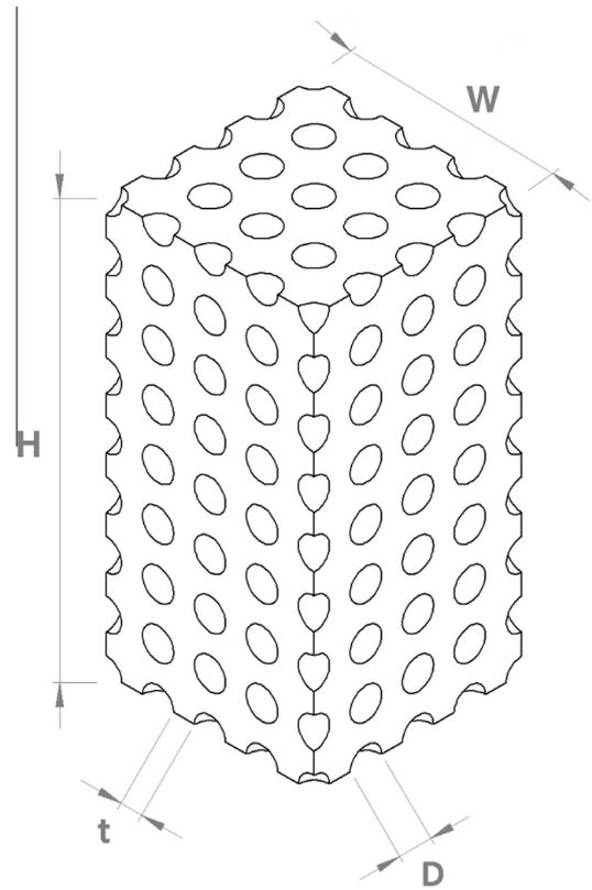
Fig. 1. The main designing parameters of tailor-made aluminum foam.
