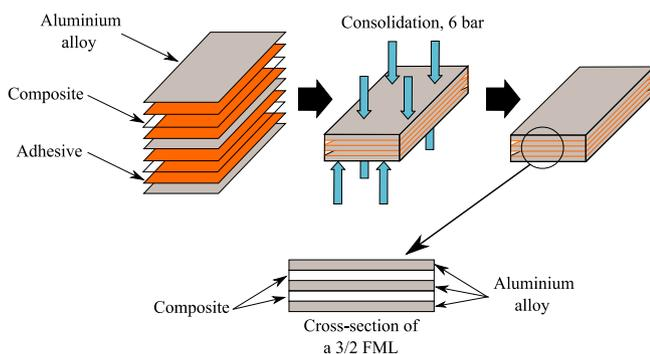
Fig. 1. FML schematic construction, adopted from [8].
