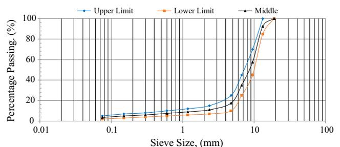
Fig. 1. Australian open graded gradation for porous asphalt mixture, (AAPA, 2004).
