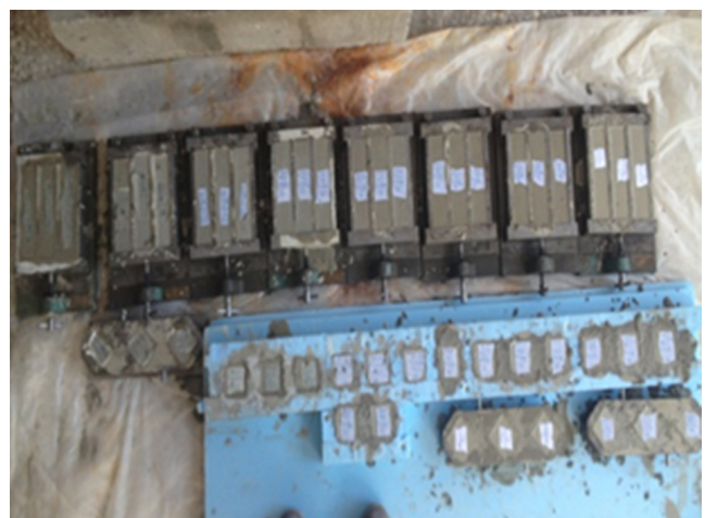
Fig. 1. Casting of 40 \times 40 \times 160 mm prismatic specimens and 50 \times 50 \times 50 mm cube specimens.
