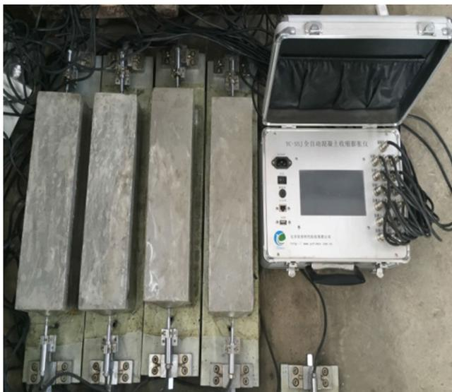
Fig. 1. Expansion test setup.
