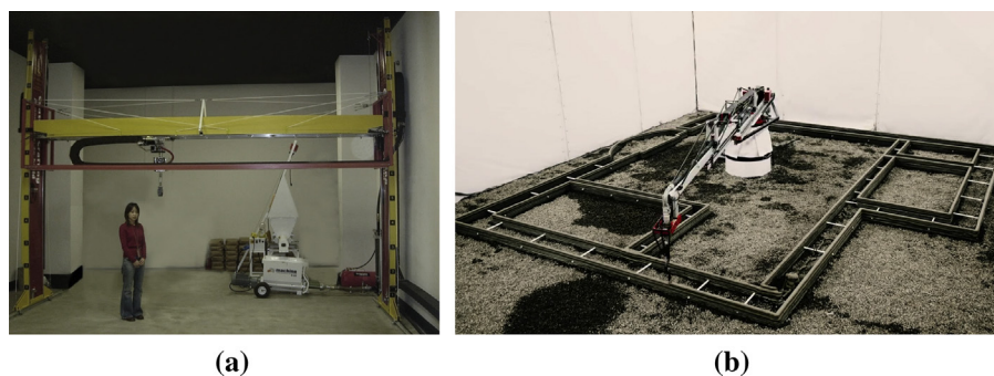
Fig. 1. (a) Contour Crafting machine (b) Crane printer developed by Apis Cor™ [22].
