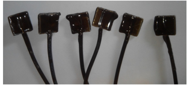
Fig. 2. The PZT electromechanical impedance sensors.
