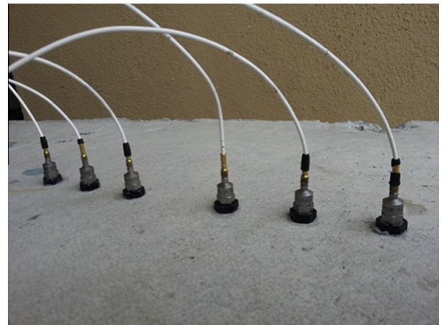
Fig. 2. Photograph of accelerometer sensors arranged on the upper side of concrete specimen.
