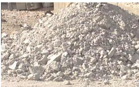
Fig. 1. Photo of chunks of concrete after crushing process.
