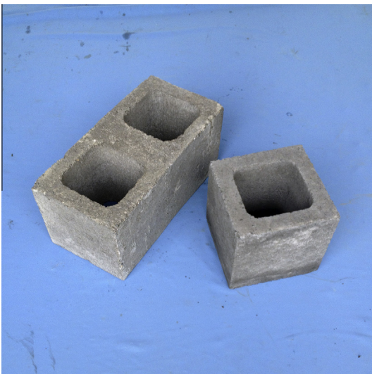
Fig. 1. Geometry of full block and half-concrete block. All masonry prisms were constructed using hollow concrete full and half blocks, the dimensions of the full and half blocks were 390 mm × 190 mm × 190 mm and 190 mm × 190 mm × 190 mm (length × height × thickness), respectively.
