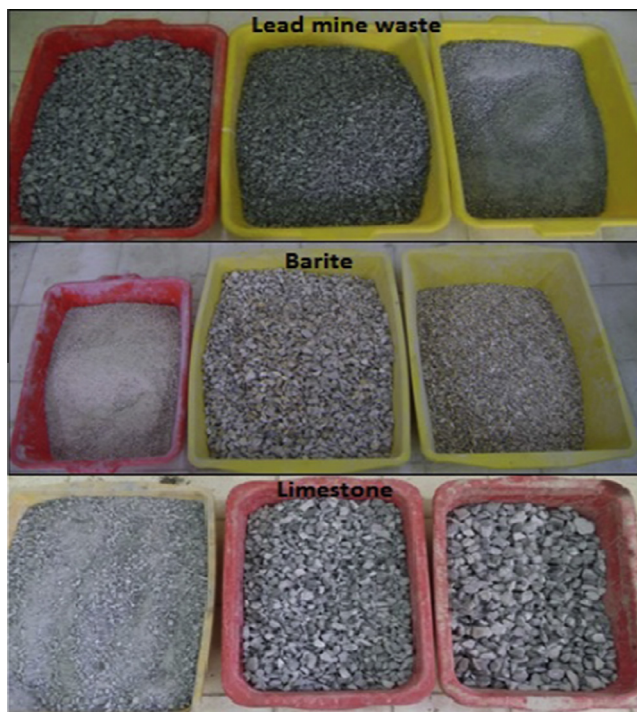
Fig. 1. Crushed aggregate in jaw broken and separated in classes.
