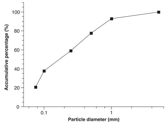
**Fig. 2.** Accumulative particle size distribution of the clayey soil.
