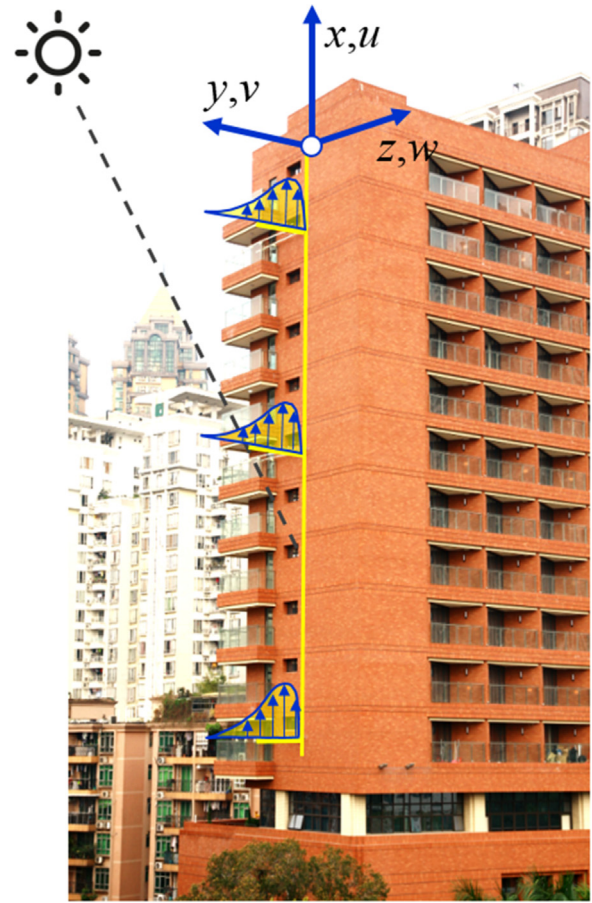
Fig. 1. Photo of the tested building and schematic of the experimental principle. x , y and z are the coordinates along the vertical wall, perpendicular to the wall and parallel to the wall, respectively. u , v and w are the velocity components in the x , y and z directions, respectively. The tested wall shown in the figure faces south.
