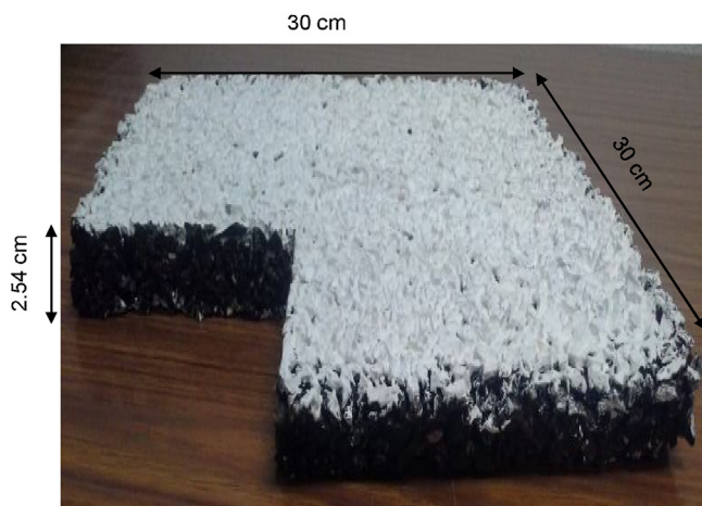
Fig. 1. Non-scaled Scrap tire block (STB) of 1 inch thickness painted white on the outer-facing surface.
