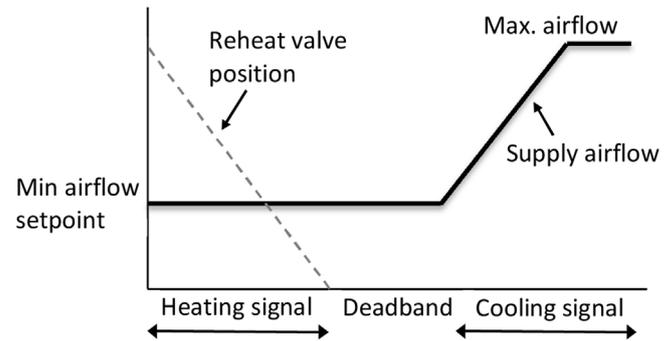
Fig. 2. Single maximum control diagram.
