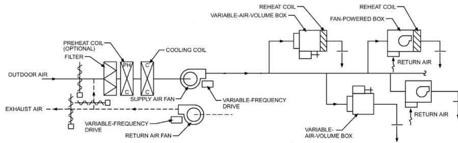
Fig. 1. Single-duct VAV system with different types of terminal units.
