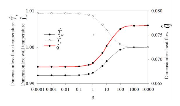
When  $\delta$  is small ( $\leq 1$ ), radiation dominates and convection has little effect. Above this value ( $\geq 1$ ), convection plays an increasing role. At the extreme limit of very large  $\delta$ , convection reaches a level such that dimensionless floor temperature  $\hat{T}_s$  and dimensionless wall temperature  $\hat{T}_w$  converge to the room temperature ( $\hat{T}_w = \hat{T}_s = 1$ ). Very high heat transfer  $\hat{q}$  from the floor is required for this limiting case.
