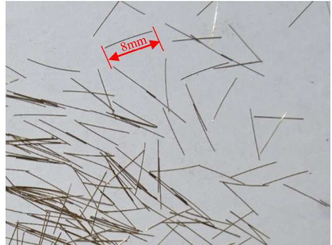
Fig. 2. Dimension of steel fibers.
