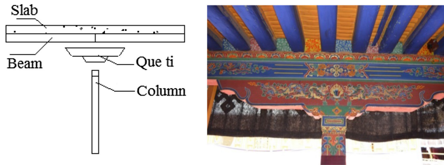
Fig. 1. The beam-column joints of typical Tibetan buildings.
