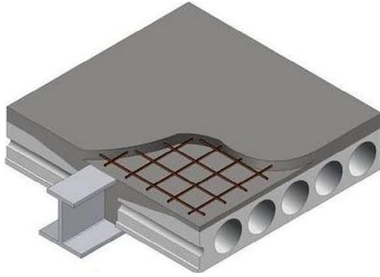
Fig. 1. Composite slim floor comprised by precast hollow core slabs and asymmetric steel beams [4].
