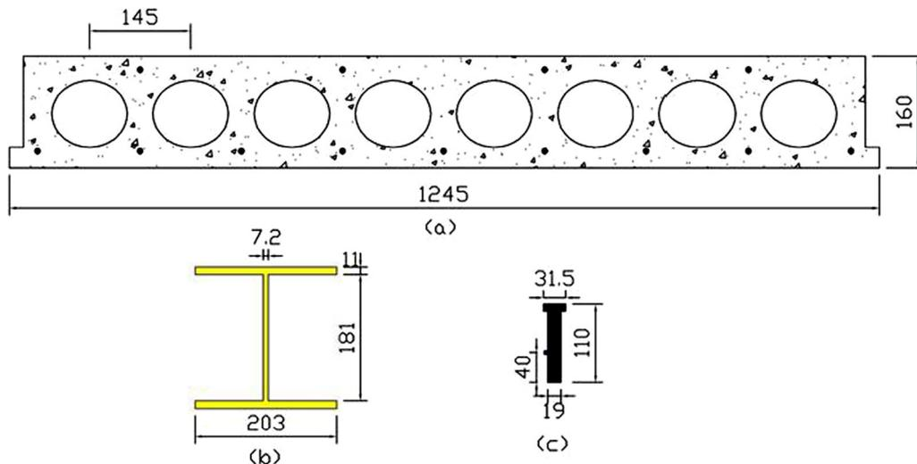
Fig. 2. Dimensions of the components of the push-out specimens (unit: millimetres).
