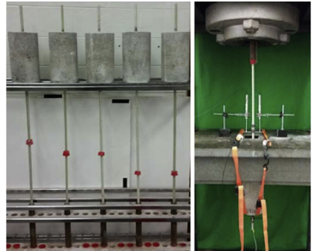
Fig. 2. A set of prepared samples (left) and complete pull-out test setup (right).
