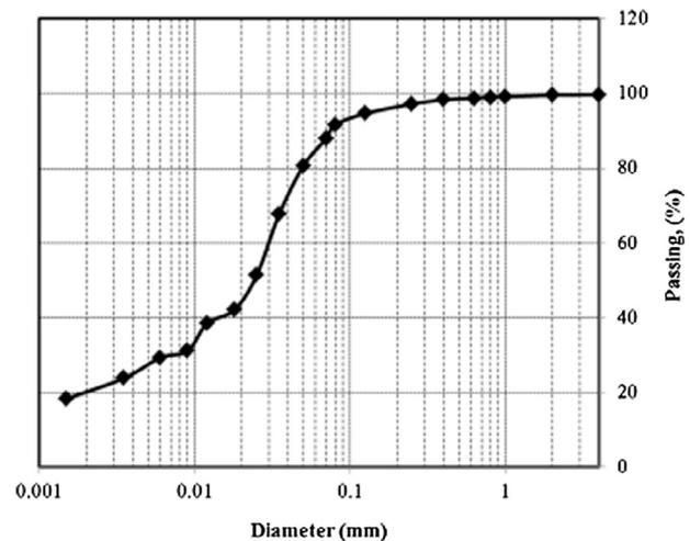
Fig. 2. Grain size distribution of the earth used.
