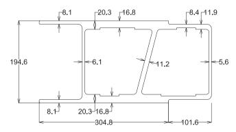
Fig. 1. Unit module geometry of DS bridge deck system; dimensions in mm.
