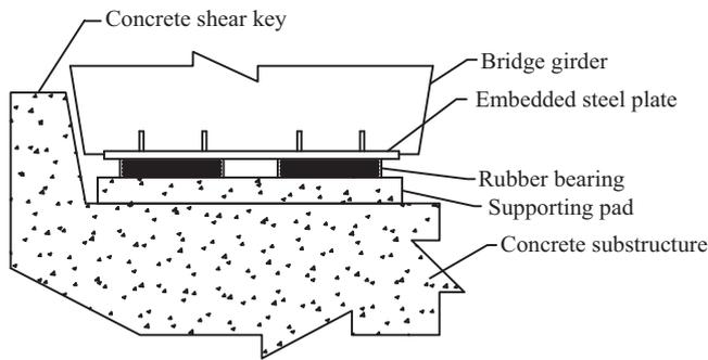
Fig. 1. Typical layout of laminated-rubber bearings.
