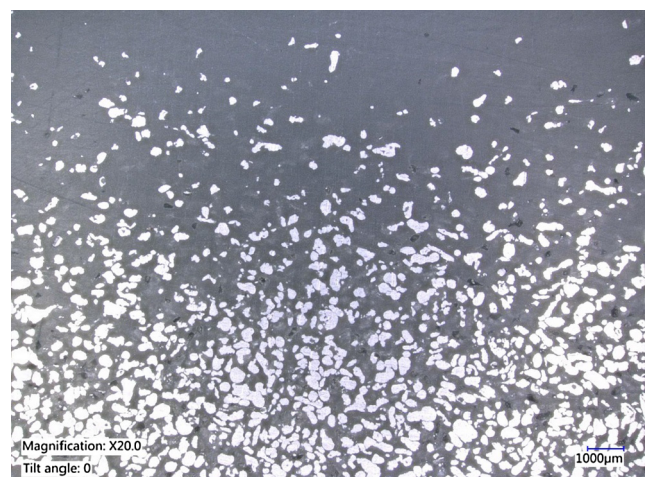
Fig. 2. Microstructure of the FGM panel containing aluminum particles dispersed in the HDPE matrix with the concentration changing in the thickness direction.
