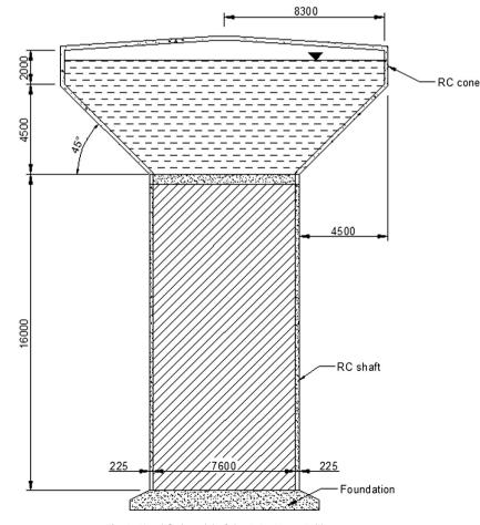
Fig. 1. Simplified model of the Anjar Nagar Palika water tower.
