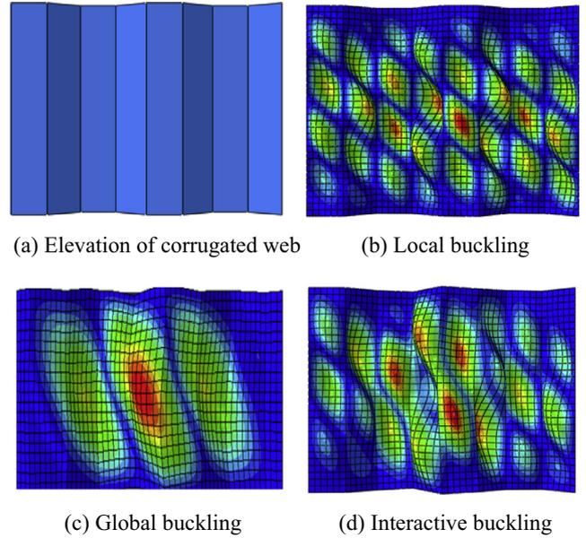
Fig. 3. Different buckling shapes in prismatic corrugated webs: (a) elevation of the corrugated web, (b) local buckling, (c) global buckling and (d) interactive buckling.
