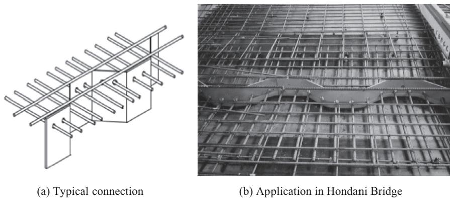
Fig. 2. Embedded connection in prestressed concrete bridges [11].
