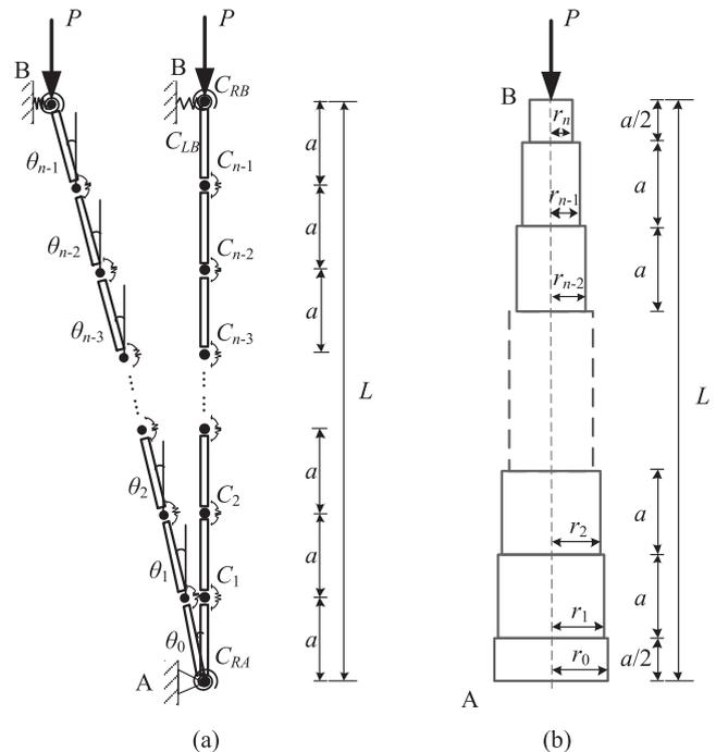
Fig. 1. (a) General HBM under axial compressive load  $P$  and (b) corresponding column shape.
