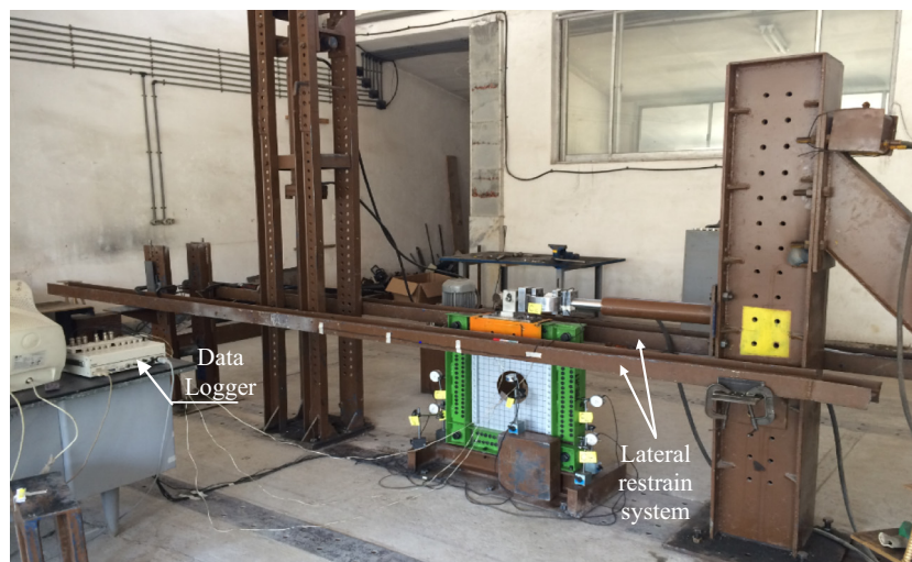
Fig. 1. Lateral restraint system of the SSSW specimens in the laboratory.
