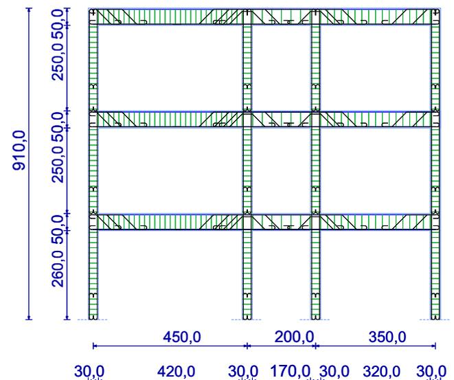
Fig. 1. Prototype RC frame, designed accordingly with the old design practice R.D. 1939. Dimensions are in millimetres.
