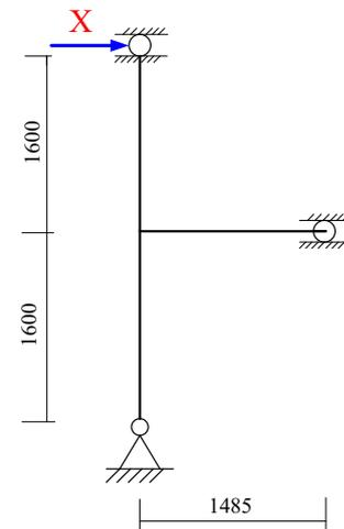
Fig. 2. General sketch of test specimens. Note: The aforementioned values respectively equal to the distances from the central point of the CFTST column to the central point of the corresponding pin.
