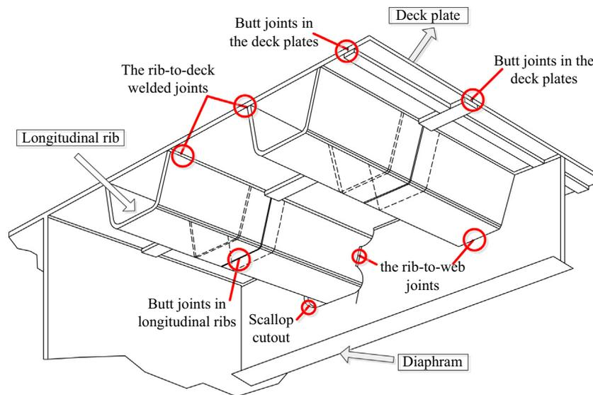
Fig. 1. Typical welded details in an orthotropic steel deck.
