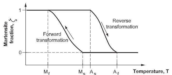
Fig. 2. Schematic phase transformation in SMAs according to temperature.
