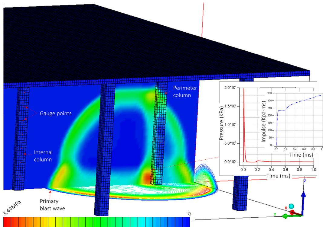
Fig. 2. Fluid-structure interaction and extracting consequential pressure histories.
