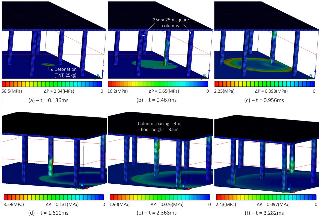
Fig. 1. CFD simulation of internal building detonation and wave propagation.
