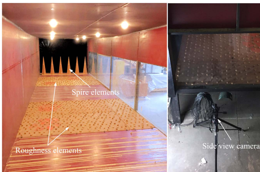
Fig. 2. (Left) Inside the wind tunnel chamber where the surface roughness elements and spire elements are installed. Also, on the right, the camera position at the side view of the release point (jet location) is shown.
