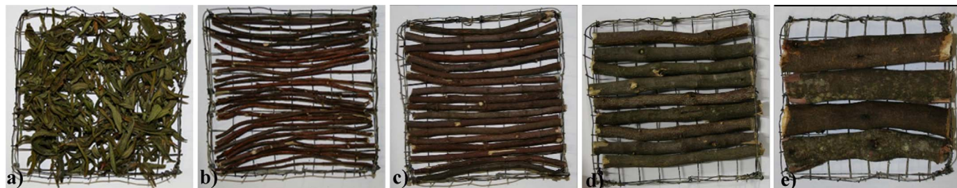
Fig. 1. Sample holder with a) leaves and twigs with diameter of b) 2 mm, c) 4 mm, d) 8 mm and e) 15 mm.
