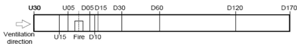
Fig. 1. Full-scale tunnel experiment instrumentation locations with upstream (U) and downstream (D) distances in metres.
