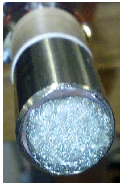
Fig. 2. Tin sample in its holder after exposure to ISTTOK plasmas.
