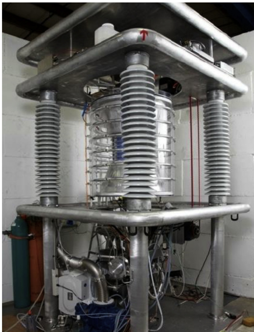
Fig. 3. Photo of SHINE neutron generator prototype.
