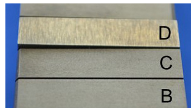
Fig. 4. Final shape of the plasma facing surface.
