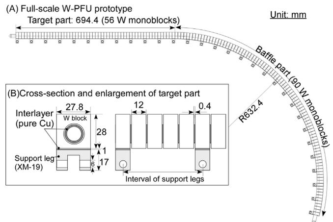
Fig. 2. Schematic drawing of full-scale W-PFU prototype.
