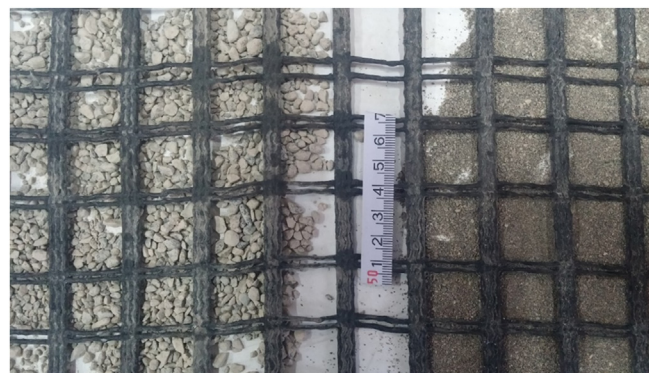
Fig. 1. A view of geogrid and sands used.
