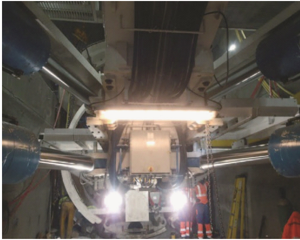
Fig. 1. Robbins Main Beam (TBM) during setup.
