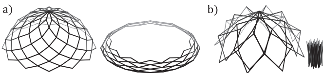
Fig. 4. (a) Single-layer scissor grid based on Hoberman's Iris dome consisting of angulated scissor units; (b) spherical double-layer scissor grid with rhomboid lamella pattern consisting of polar scissor units and based on Escrig (1985).
