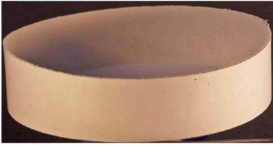
Fig. 1. Geometry of the deep-drawn paperboard in use for new packaging applications with a diameter of 100 mm and a height of 25 mm, cf. Hauptmann and Majschak (2011).
