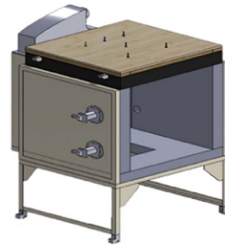
Fig. 2. Wooden slab set up in the fire resistance furnace.
