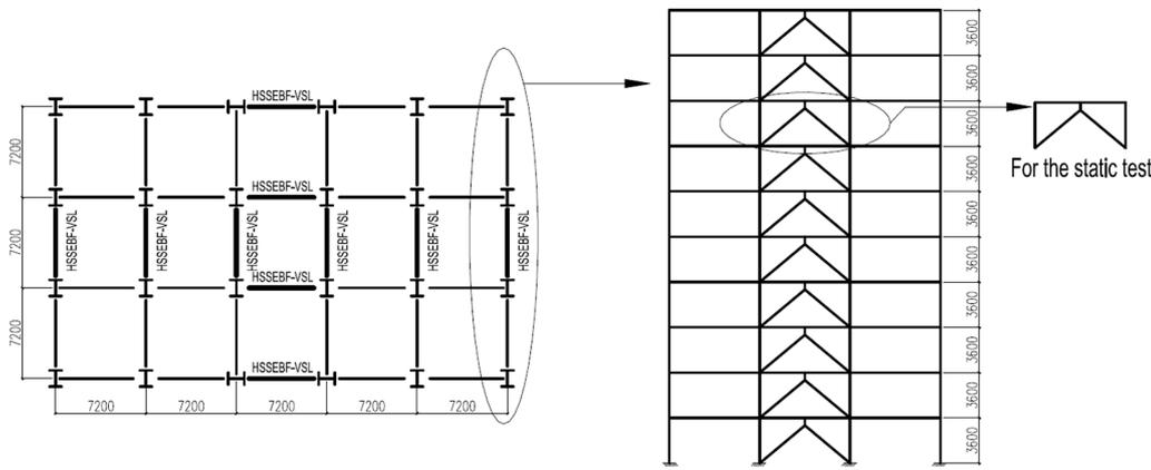
Fig. 1. Prototype structure for static tests.
