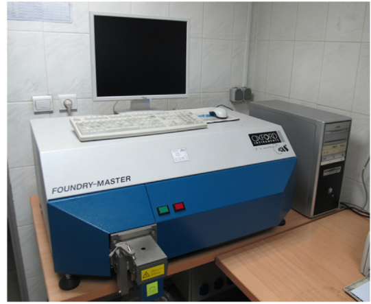
Fig. 1. FOUNDRY-MASTER UV metal analyzer.
