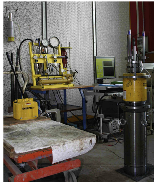
Fig. 1. Cutaway section of the pull-out bench and overview of the laboratory facility.
